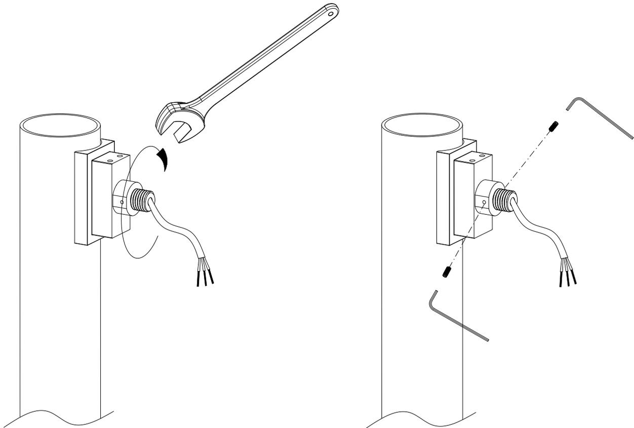
**3** Refer to the wiring diagram for wiring and secure the fixture
